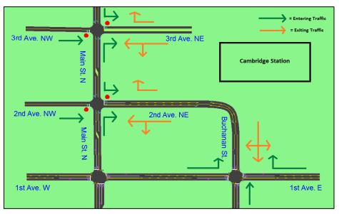
Figure 3-12: Cambridge Station Entering and Exiting Turning Movements
