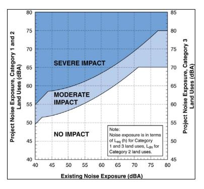
Figure 4-4: Noise Impact Criteria for High Speed Rail Projects
